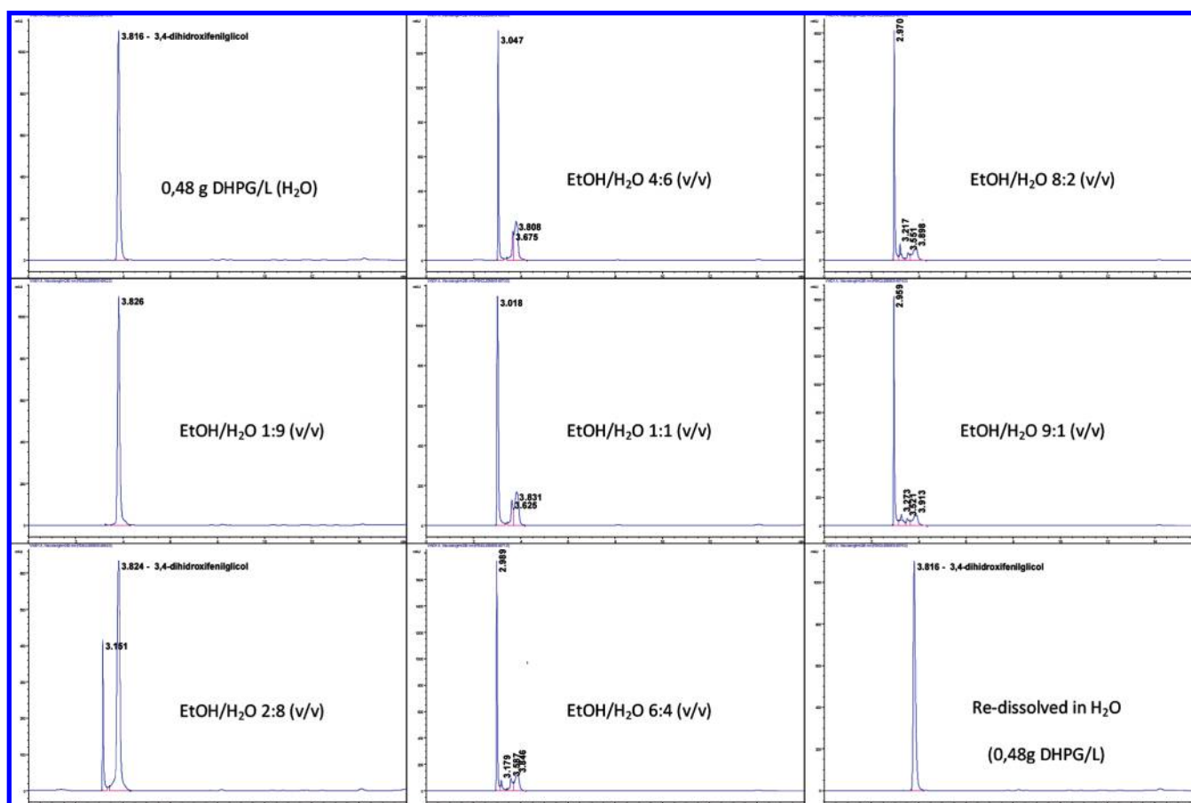
Figure 2. HPLC chromatograms at 280 nm of pure dihydroxyphenylglycol (DHPG) in ethanolic solutions: evolution of DHPG peak to increasing concentrations of ethanol and when redissolved in water.
